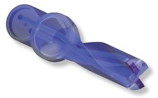
Twisted coolant hole in the drill body increases coolant flow by 1.5 times, which improves chip evacuation, resulting in excellent surface finish.
